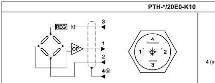
1 = output 0 ÷ 10 V 2 = 0 V 3 = 12 ÷ 30 VDC 4 (indicated on the connector by the symbol  $\bigoplus$  = GND
