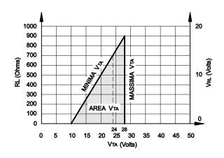
N.B. Outside the VTA area the correct functioning of the transducer is not assured.
