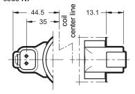
connection for DUAL DIN 43650 connector type code **K12**
