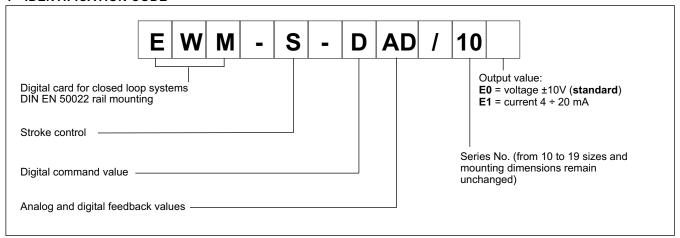
The card EWM-S-DAD is an evolution of an analog model (EWM-S-AD). The customer can choose between two sensor types: analog or digital and the communication with the PLC is via Profibus DP.
