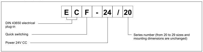
The ECF connector is a digital amplifier controlling open loop on-off valves.
