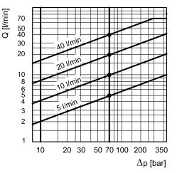
The diagram states the maximum valve controlled flow rate according to the pressure drop between the P and T ports.
